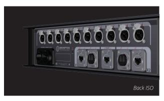
Additional **XD** units can be daisy-chained together to extend the signal, allowing screens in different locations to be connected to a single 10G trunk. All ten 1G outputs on each **XD** can be used, as long as the combined pixel load on all ports of the same number does not exceed the pixel capacity of a single 1G link.
